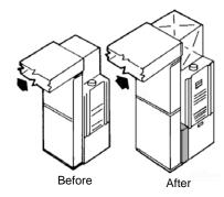
Offset Installation—If there is less than 7-in. for mounting the air cleaner between the duct and the furnace, move the return air drop.
